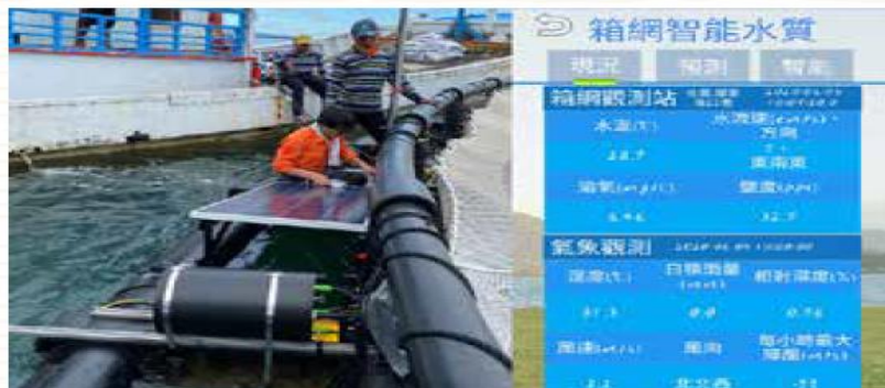
Smart net cage aquaculture monitoring system equipment and App interface
